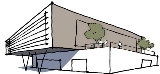
Overhangs provide shade and shifts in building massing create second-story terraces.
